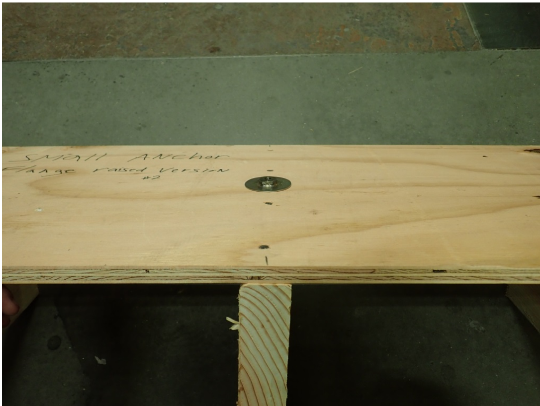
Photo 8 – Overview of the NB2 (Small Anchor Flange Raised) configuration.
