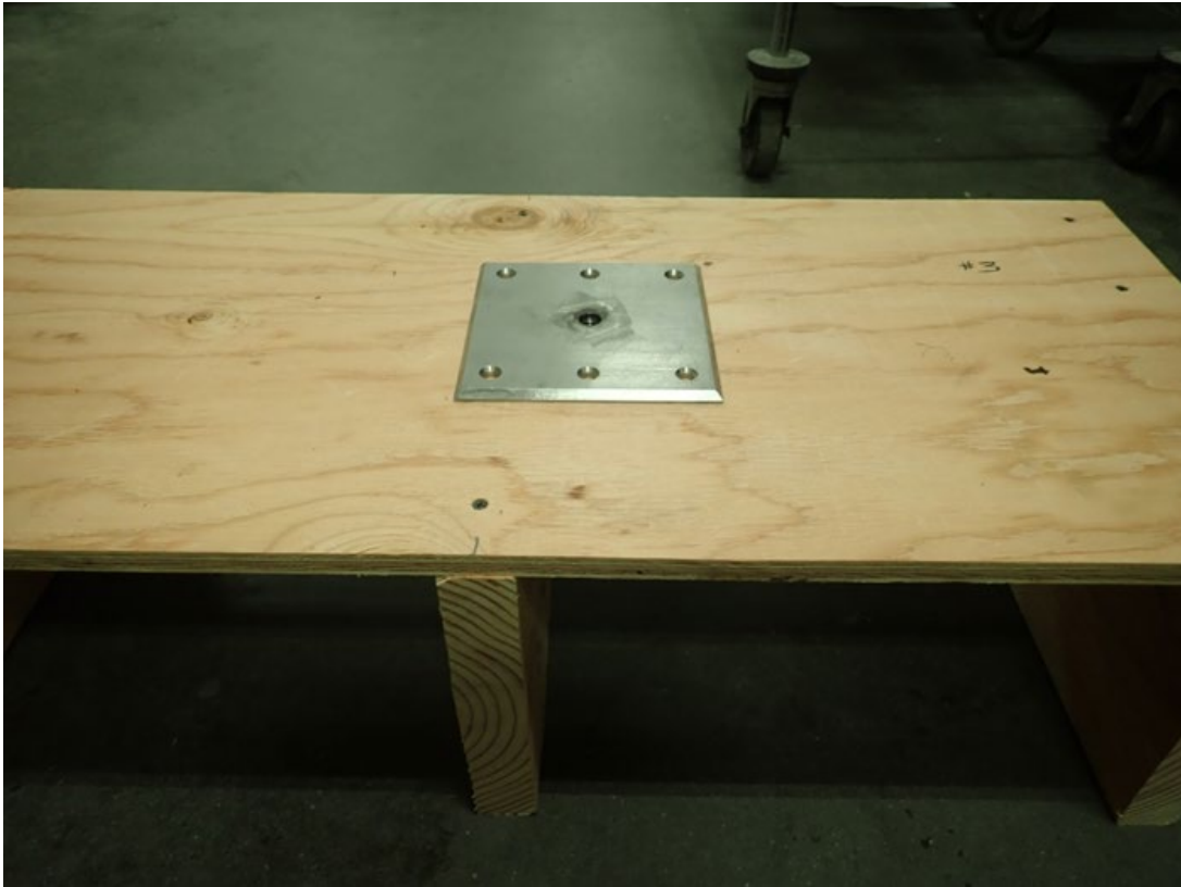
Photo 5 – Overview of the NB1C (Flush Anchor, 3/4 in Bolt) configuration.
